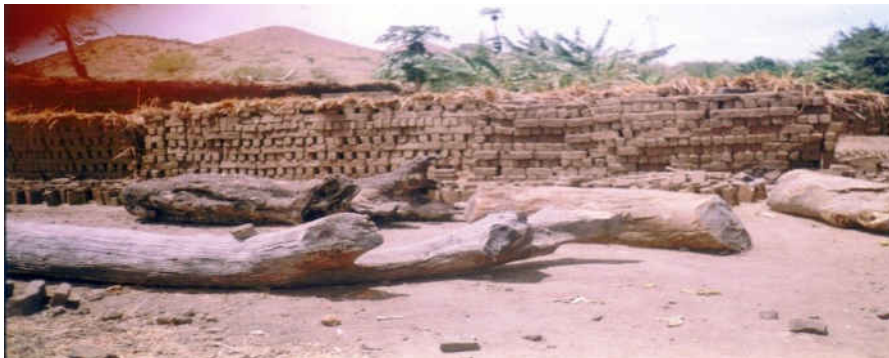
Plate 7: A bundle of un-burnt bricks and logs for burning the bricks
