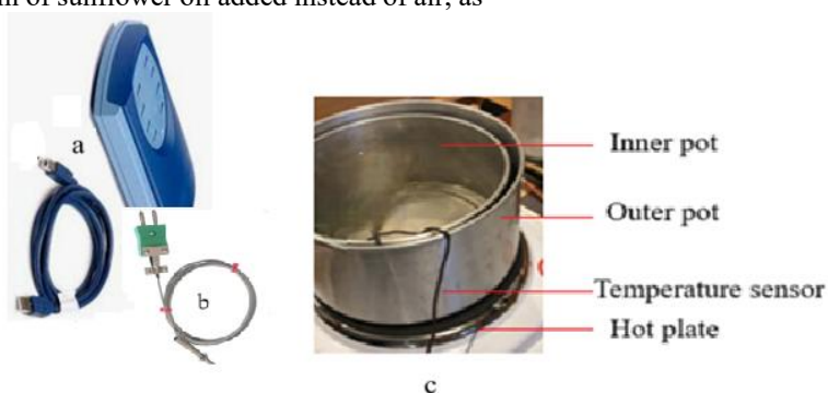
Figure 3: Image showing: TC-08 data logger, (a), k-type thermocouple sensors (b), and the arrangement of pots for both aluminium and stainless steel referred to as pot in pot (a) whereby one pot is inserted inside the other.
